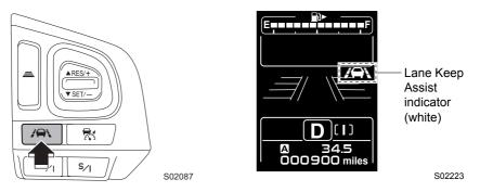
Press the (Lane Keep Assist) switch once again to turn it off, and " (Lane Keep Assist indicator) is turned off on the EyeSight display area.
