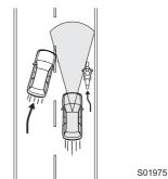
When driving on curved roads, at the start and end of a curve and on roads continuous curves (These conditions make it difficult for the system to detect vehicles because outside the they are detectable area.)
