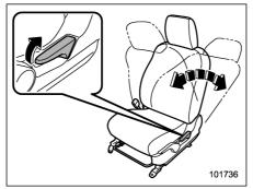
Pull the reclining lever up and adjust the seatback to the desired position. Then release the lever and make sure the seatback is securely locked into place.
