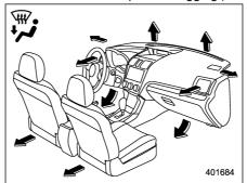
(Heat-def): Windshield defroster outlets, foot outlets and both side outlets of the instrument panel (Refer to "Defrosting" \$\tilde{\pi}\$4-11.)
