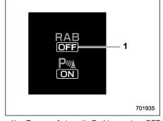
Reverse Automatic Braking system OFF indicator
