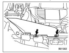
To replace the right side headlight bulb, use a screwdriver to undo the clips on the air intake duct, then remove the air intake duct.
