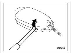
2. Carefully pry the remote engine start transmitter halves apart using a small flathead screwdriver.
