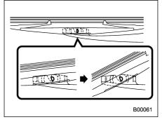
2. Turn the wiper blade assembly counterclockwise.
