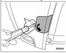
2. Cover the tip of a flat-head screwdriver with vinyl tape or cloth so that it will not scratch the bumper. Insert the flat-head screwdriver into the cutout of the cover and pry open the cover.
