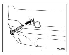
3. Screw the towing hook into the thread hole until its thread can no longer be seen.
