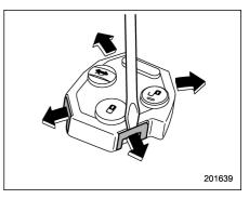
3. Open the transmitter case by releasing the hooks.
