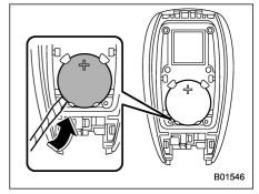
3. Take out the battery using a flat-head screwdriver with vinvl tape or a cloth.
