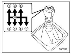
This manual transmission is a completely synchromesh, 6-forward-speed and 1-reverse-speed transmission.
