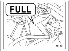
Remove the washer tank filler cap, then add windshield washer fluid until it reaches the "FULL" mark on the tank. If windshield washer fluid is unavailable use clean water.
