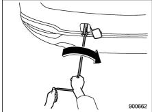
4. Tighten the towing hook securely using the jack handle.
