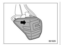
2. Slide the rear combination light assembly rearward and remove it from the vehicle.
