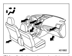
(Bi-level): Instrument panel outlets and foot outlets
