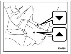
4. After fastening the seatbelt, make sure that the "\(\nblue\)" mark on the connector (tongue) and the "A" mark on the buckle face outwards.
