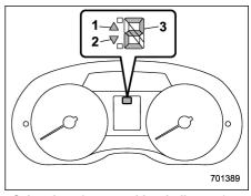
Select lever/gear position indicator (type A)
