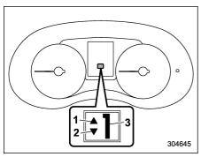
Select lever/gear position indicator (type B)
