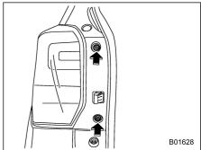
7. Tighten the upper and lower screws.
