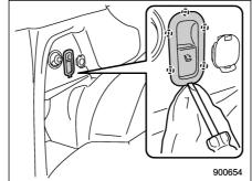
1. Release the fitting on the left side rear seat release latch.
