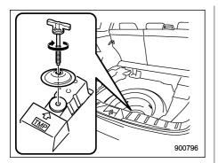
17. When storing the spare tire after repairing a flat tire, be sure to place the spacer in the manner shown in the illustration, and then tighten the bolt in the rear side of the bracket.
