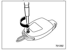
1. Remove the small phillips screw located on the back side of the transmitter.
